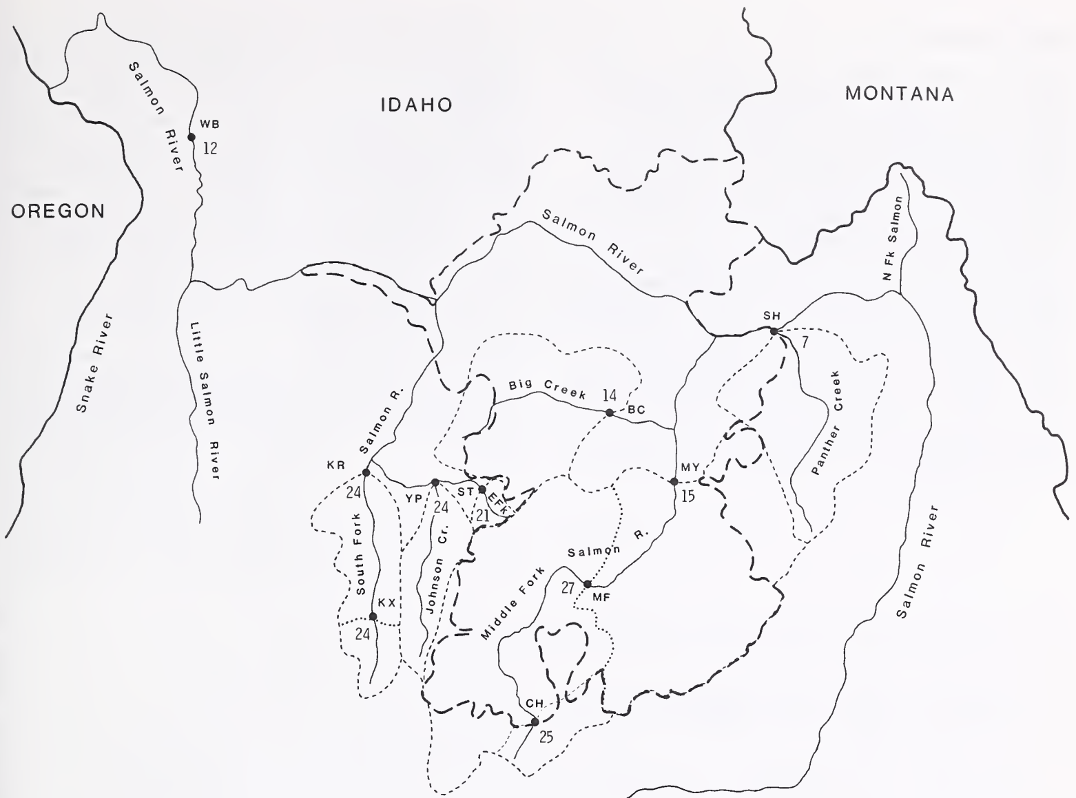
Figure 14—Average yearly runoff, equivalent depth in inches, from drainages or subdrainages in or adjacent to RNR (boundary shown by heavy dashed line). Drainage areas, above gauging points (heavy dots), are shown within fine-dashed or dotted lines. EFK denotes East Fork of South Fork Salmon River. Gauging points are identified in table 11 (appendix). Runoff value at White Bird (WB) is for overall 13,550-mi 2 drainage area of Salmon River.
